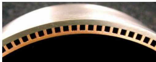
Figure 1-3: Typical cross section showing copper alloy inner liner with milled out channels and applied nickel alloy outer jacket. Obtained from [4].
