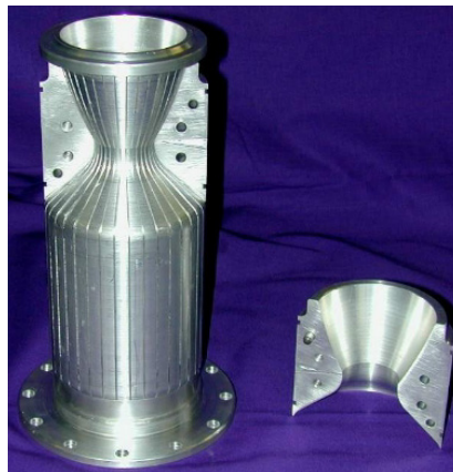
Figure 1-2: Typical milled out liquid rocket engine cooling channel application on the inner liner with detached outer jacket portion. Obtained from [4].
